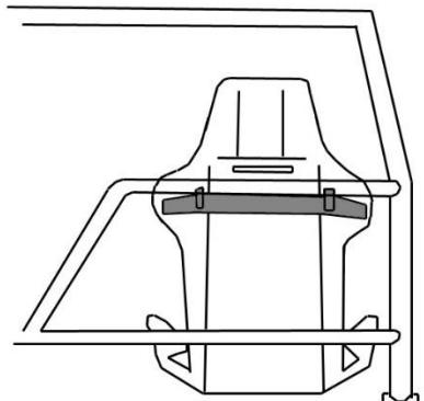
You may fit a Head Restraint Net on the on the safety fence side of the race car only. A quick release window net must be fitted to the driver's door window aperture and must be of quick release/cloth type only. Net spacing must be 76mm x 76mm maximum.
